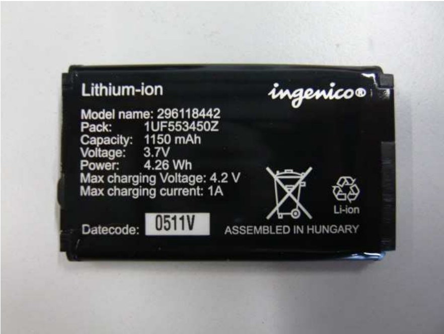
General view of Battery pack
