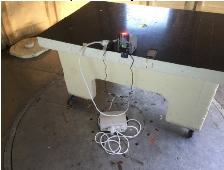
General Test setup on OATS worst case presented (30MHz to 1GHz, configuration 1, same setup for configuration 2)
