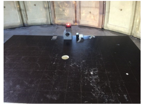
General Test setup on OATS worst case presented (30MHz to 1GHz, configuration 1, same setup for configuration 2)
