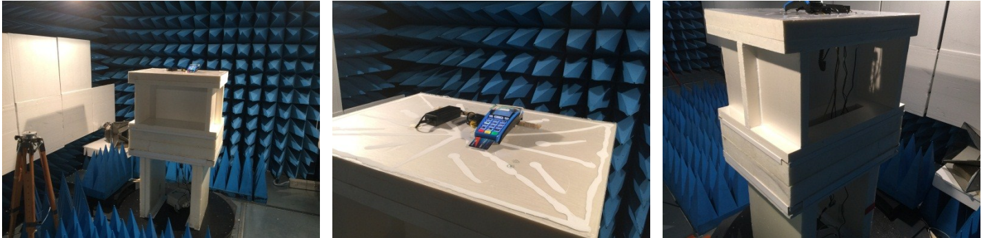
Test setup in anechoic chamber (1GHz to 2GHz)
