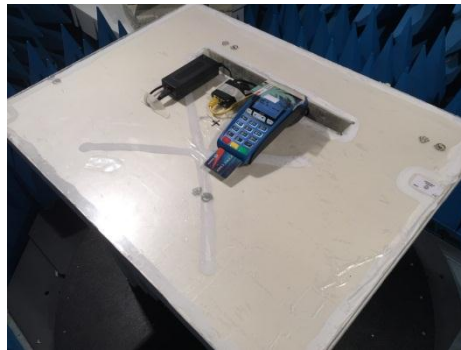
Test setup in anechoic chamber (9kHz to 1GHz)
