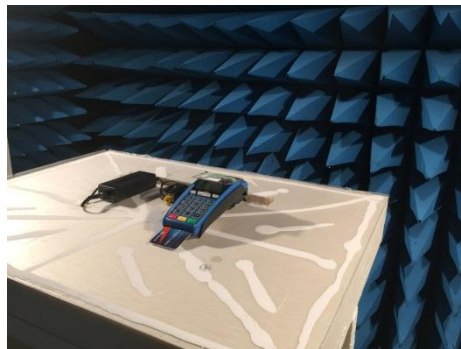
Test setup in anechoic chamber (1GHz to 2GHz)
