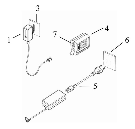
Plug: TNV-3 circuit: Telecommunication Network Voltage, as per safety standard EN 60950.
