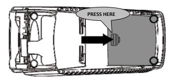
Insert the SAM Card into the slot marked (1) or(2). Take care to ensure that the SAM Card is inserted in the correct manner. The cut corner must be positioned as indicated on the figure.
