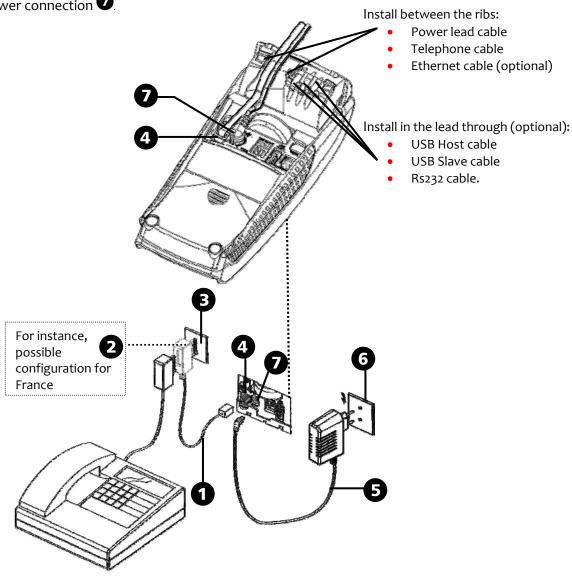
Plug: TNV-3 circuit: Telecommunication Network Voltage, as per safety standard EN 60950.
