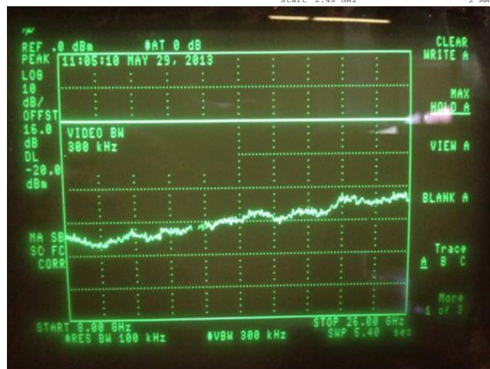
Measurement from 8GHz to 26GHz: No frequency observed
