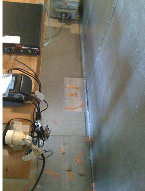
Conducted emission test setup for all configurations
