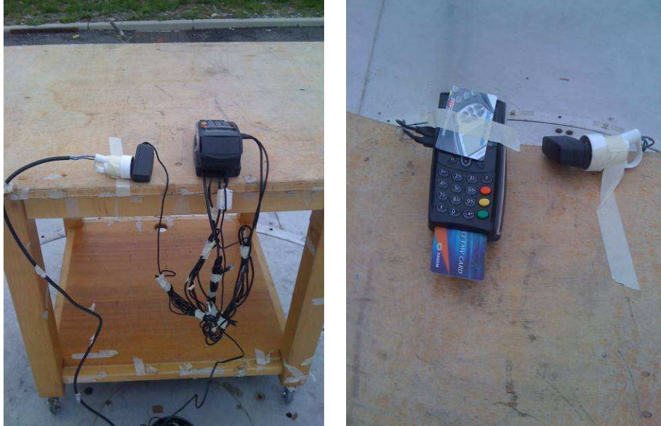
Radiated emission test setup for all configurations
