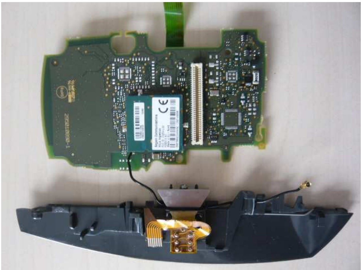
Detail views PCB of terminal
