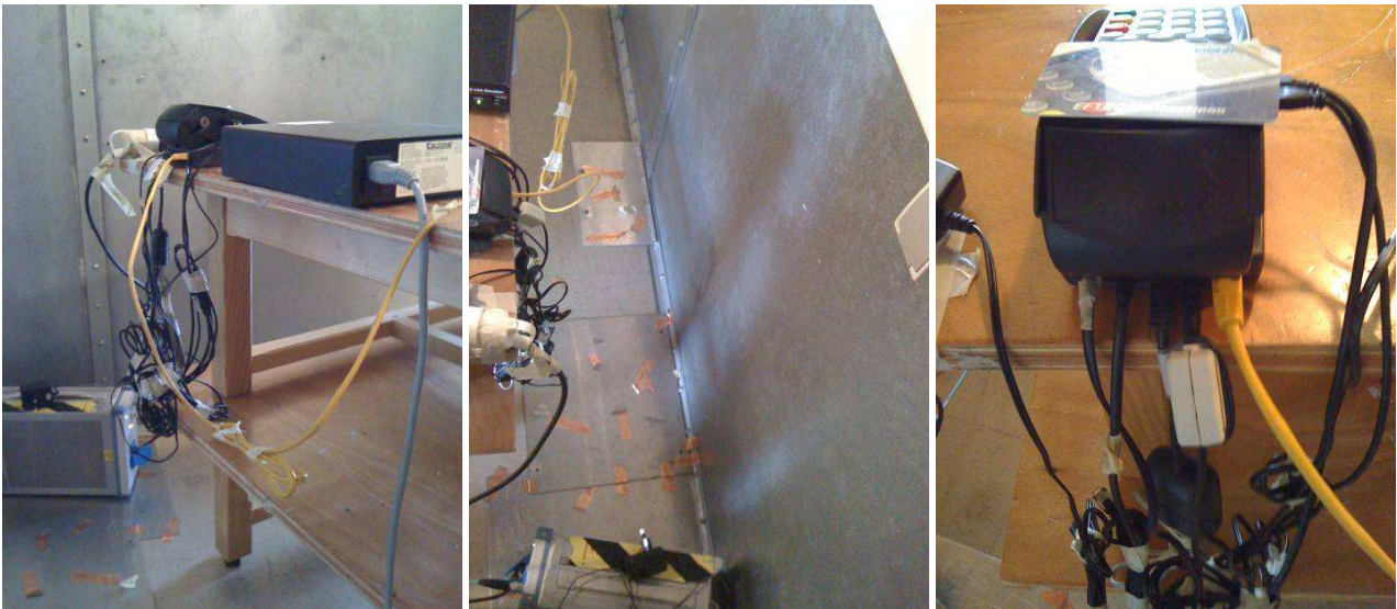
Conducted emission test setup for all configurations
