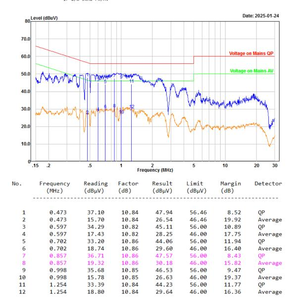
Project No.: 2402Y99420E-RF-A1 Port: neutral Test Mode: Transmitting IF B/W 9kHz PK/AV Serial No.: 2TOQ-1 Tester: Yukin Qiu
