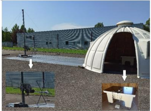
Photo Setup – OATS (Bilog antenna)
