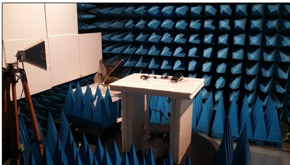
Test setup in anechoic chamber (Configuration n°1)
