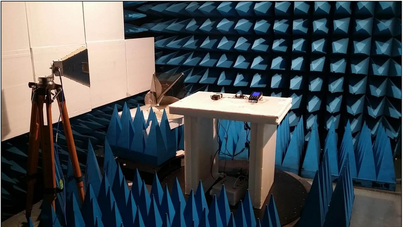
Test setup in anechoic chamber (Configuration n°8)
