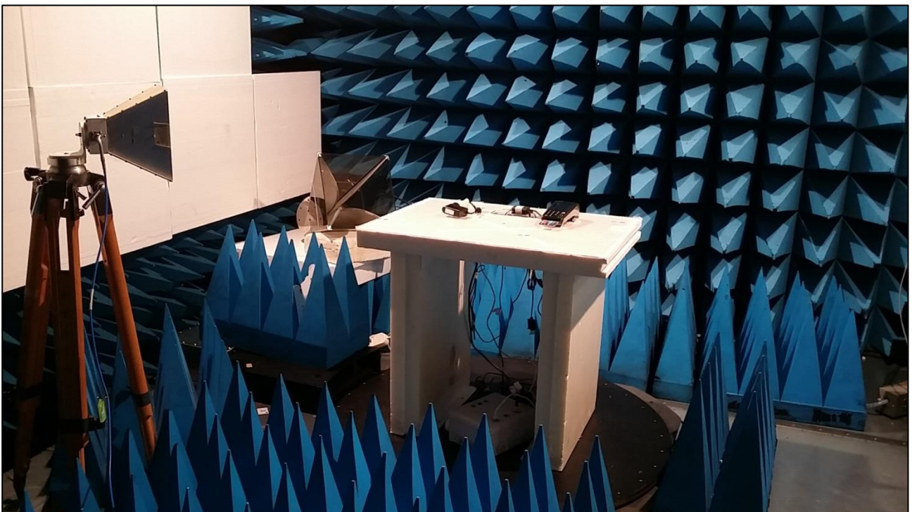
Test setup in anechoic chamber (Configuration n°2)
