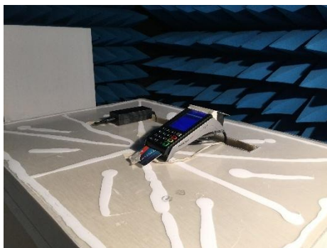
Test setup in anechoic chamber (Above 1GHz)
