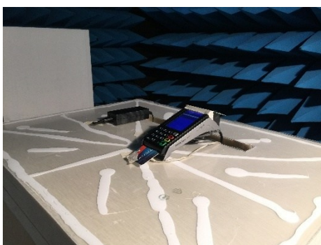
Test setup in anechoic chamber (Above 1GHz)
