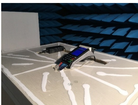
Test setup in anechoic chamber (Above 1GHz)
