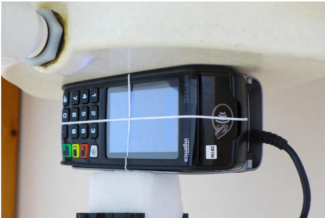
Pic. 4: Test position – left side, 0mm distance to phantom.
