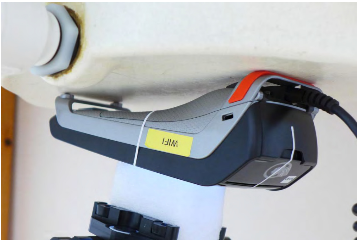
Pic. 5: Test position – back side, 0mm distance to phantom.
