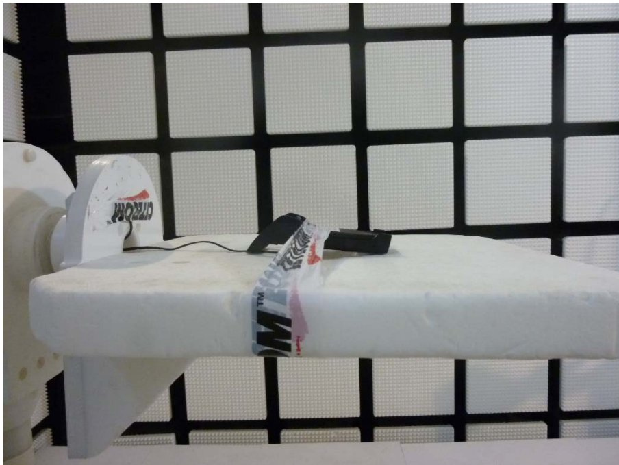
Photo 2: EUT at the anechoic chamber
