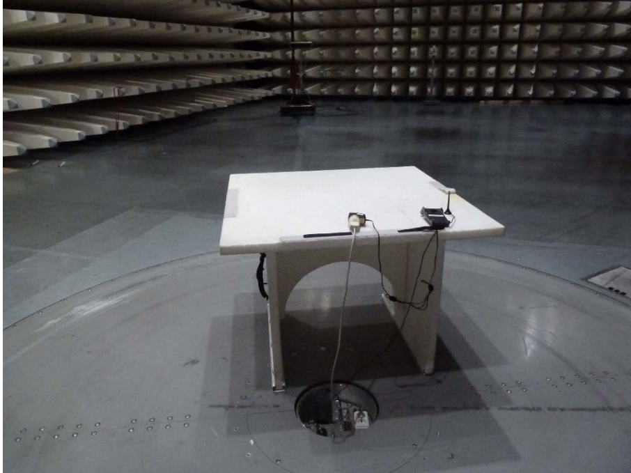
Photo 9: EUT at the semi-anechoic chamber
