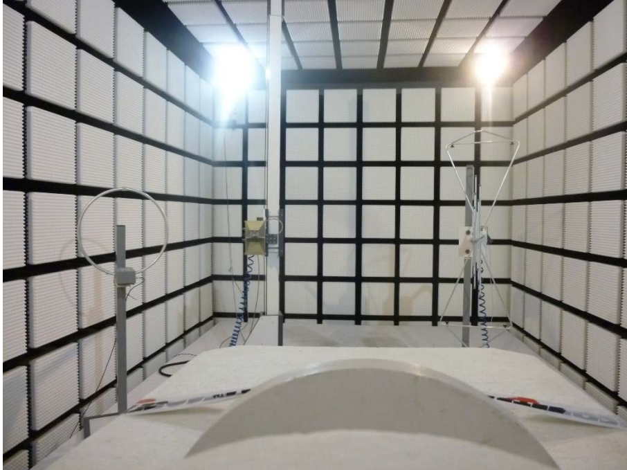
Photo 3: EUT at the anechoic chamber
