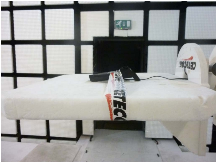
Photo 4: EUT at the anechoic chamber
