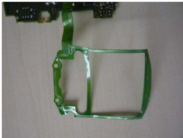
Detail views 13.56MHz antenna
