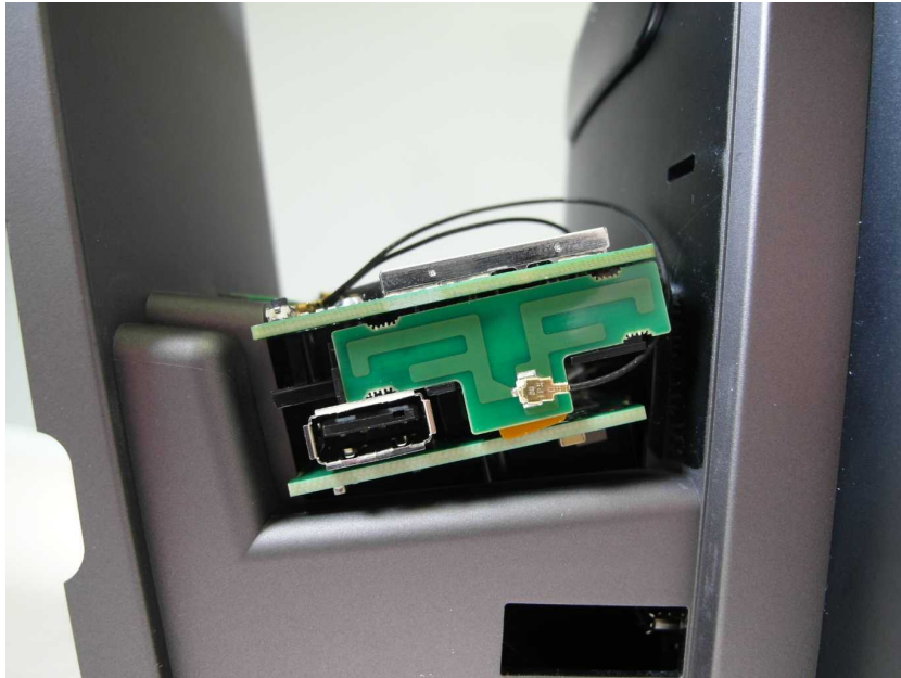
Photo 9: Antenna: Antenna, front side view
