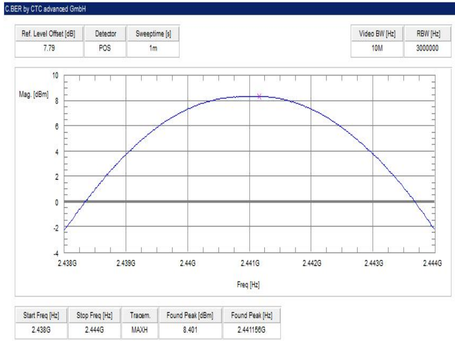
Plot 5: middle channel – 2441 MHz, Pi / DQPSK modulation
