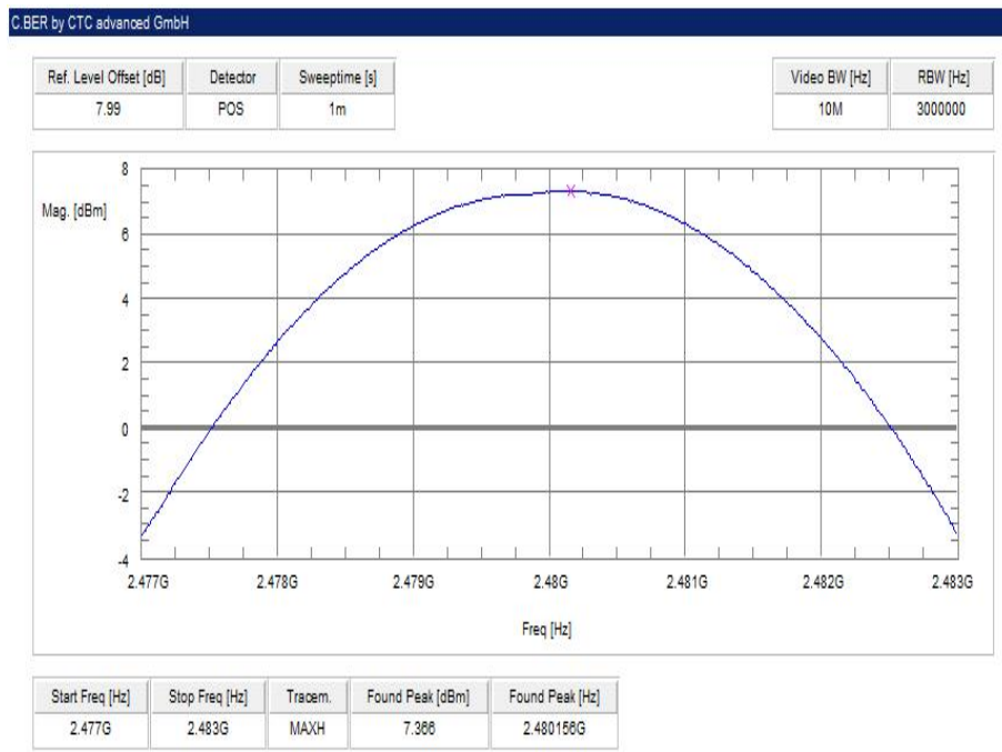
Plot 6: highest channel – 2480 MHz, Pi / DQPSK modulation
