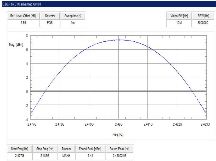
Plot 3: highest channel – 2480 MHz, GFSK modulation
