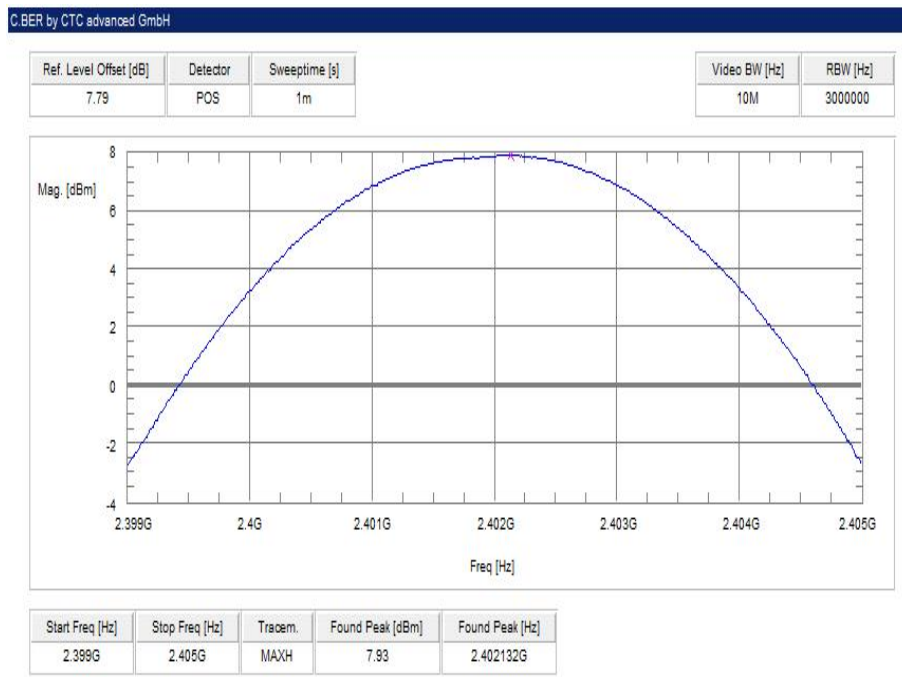
Plot 4: lowest channel – 2402 MHz, Pi / DQPSK modulation
