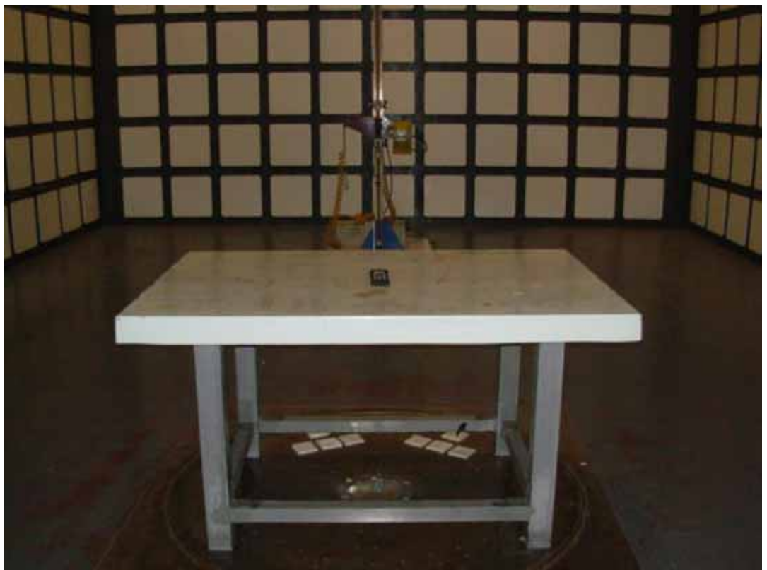
BACK VIEW OF TEST (ABOVE 1GHZ, LYING DIRECTION)
