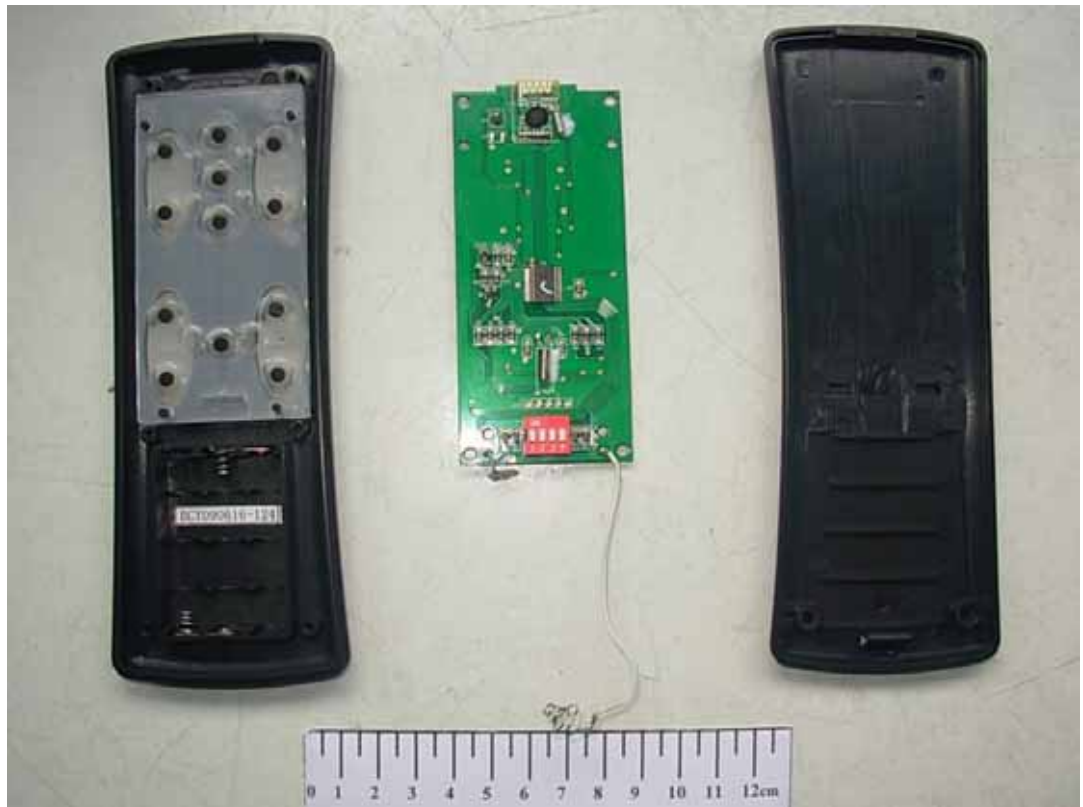
FIGURE 1 REMOTE CONTROLLER (M/N: BCYK001) COVER REMOVED
