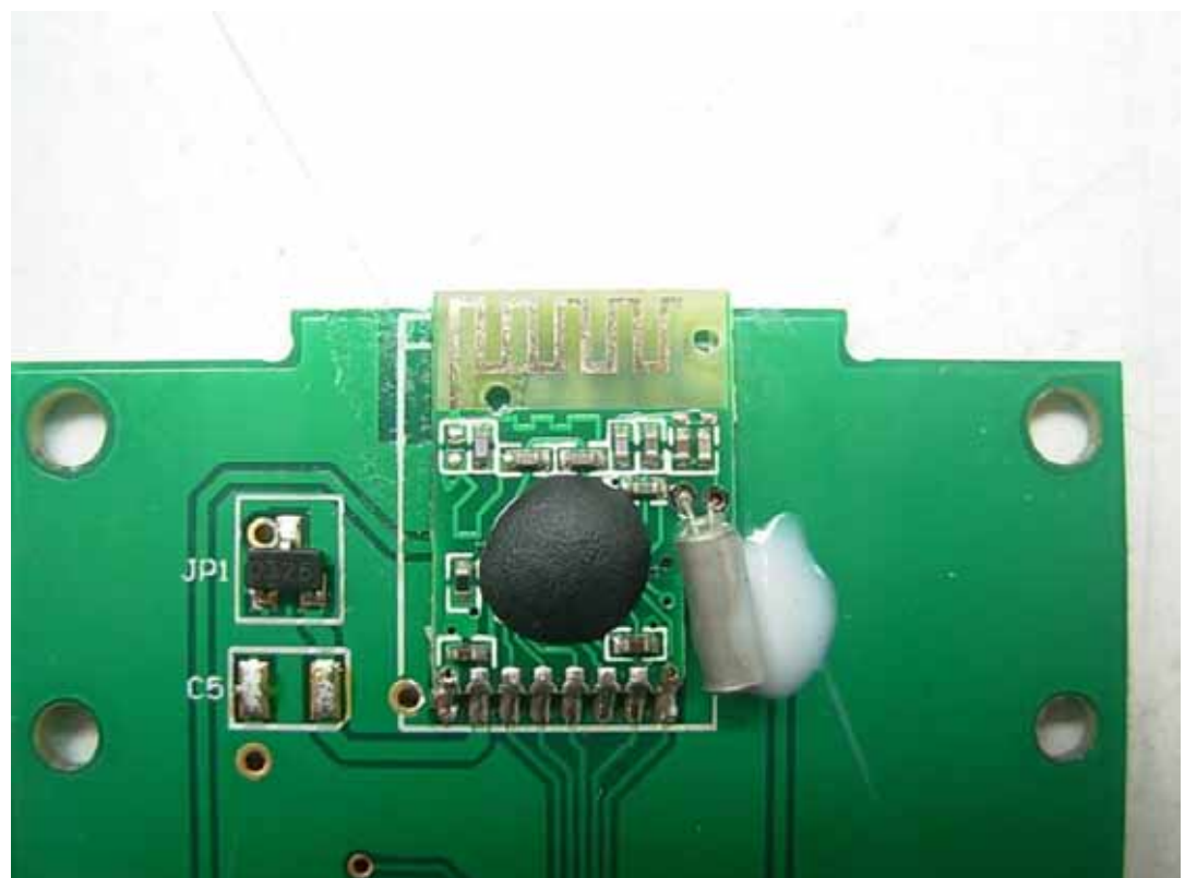
FIGURE 4 REMOTE CONTROLLER (M/N: BCYK001) RF MODULE
