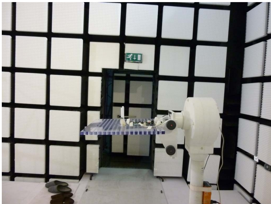
Photo 4: EUT with internal antenna in the anechoic chamber
