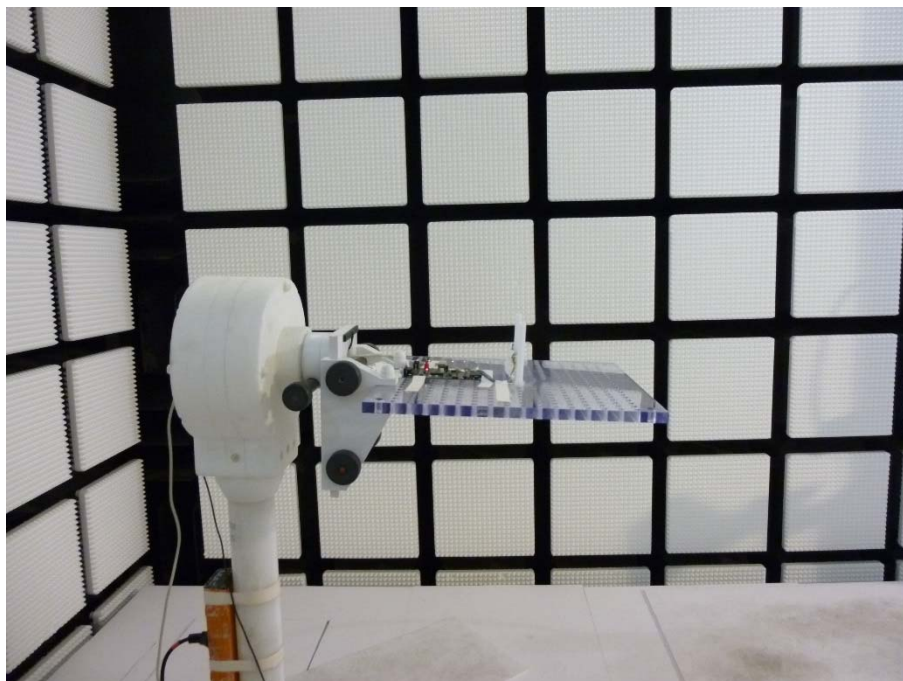
Photo 2: EUT with internal antenna in the anechoic chamber
