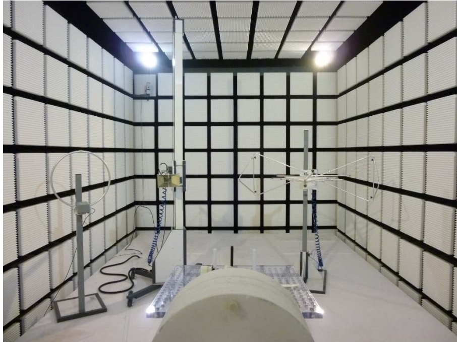
Photo 11: EUT with external rubber antenna in the anechoic chamber
