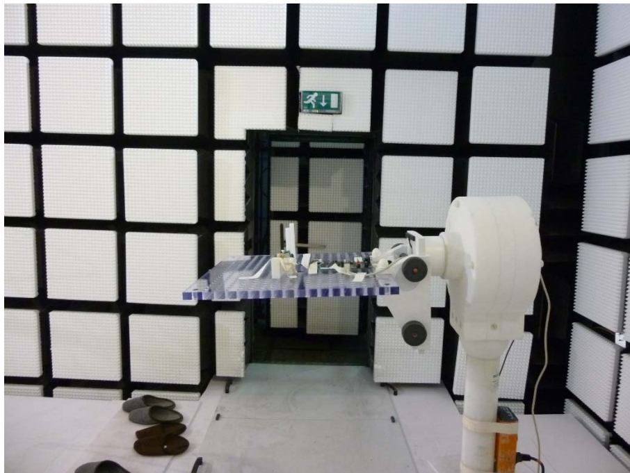
Photo 12: EUT with external rubber antenna in the anechoic chamber
