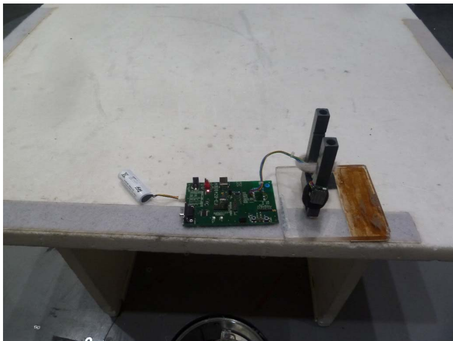
Photo 8: EUT with internal antenna in the semi-anechoic chamber
