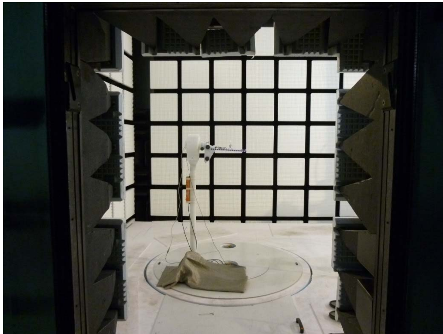
Photo 22: EUT with external PCB antenna in the anechoic chamber
