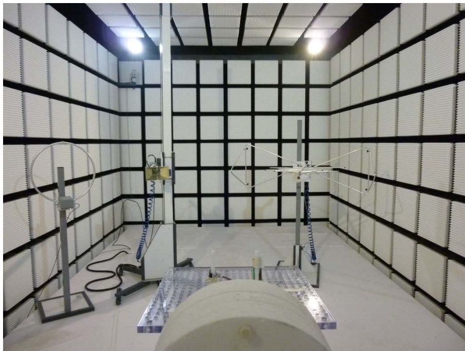
Photo 18: EUT with external PCB antenna in the anechoic chamber
