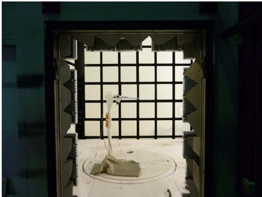
Photo 1: EUT with internal antenna in the anechoic chamber
