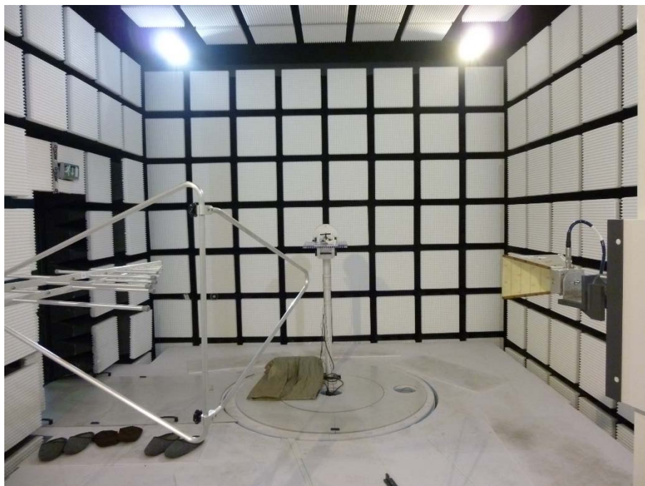
Photo 14: EUT with external rubber antenna in the anechoic chamber
