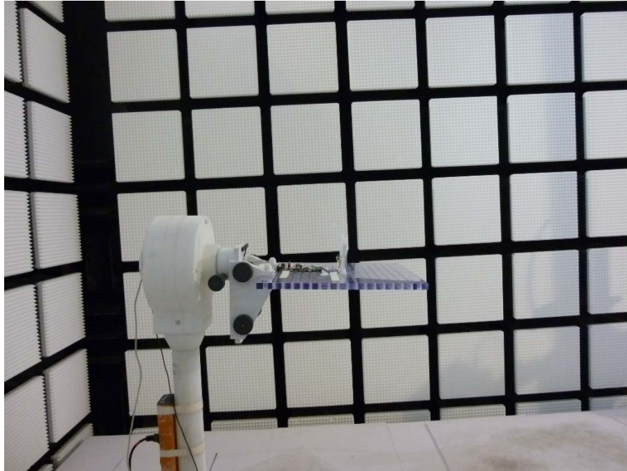
Photo 17: EUT with external PCB antenna in the anechoic chamber
