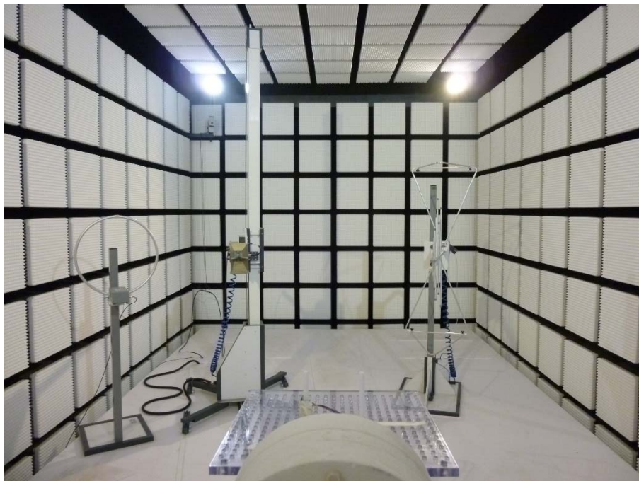
Photo 3: EUT with internal antenna in the anechoic chamber
