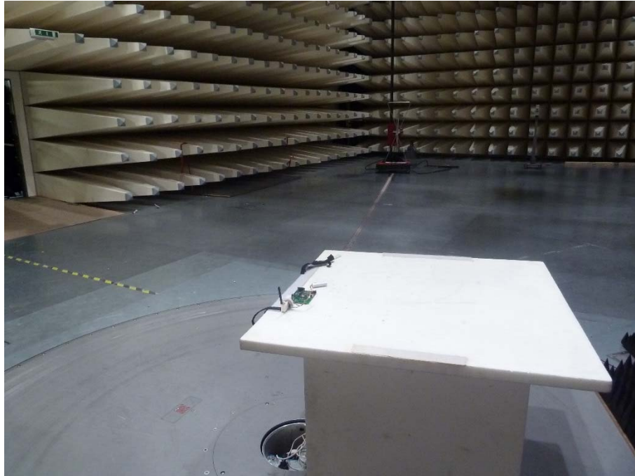
Photo 15: EUT with external rubber antenna in the semi- anechoic chamber
