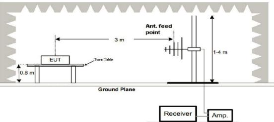
3. Radiated Emission Test-Up Frequency Above 1GHz
