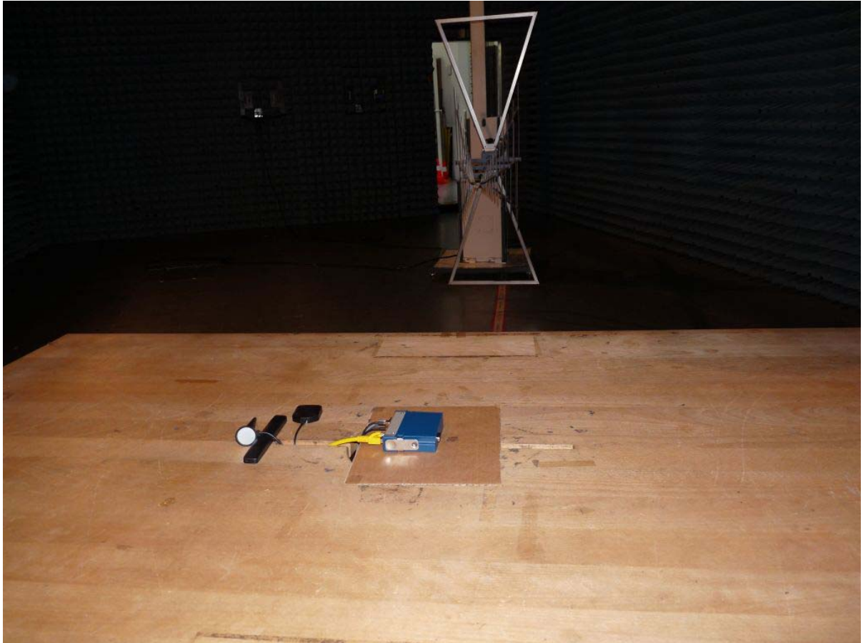
setup for the test radiated emissions
