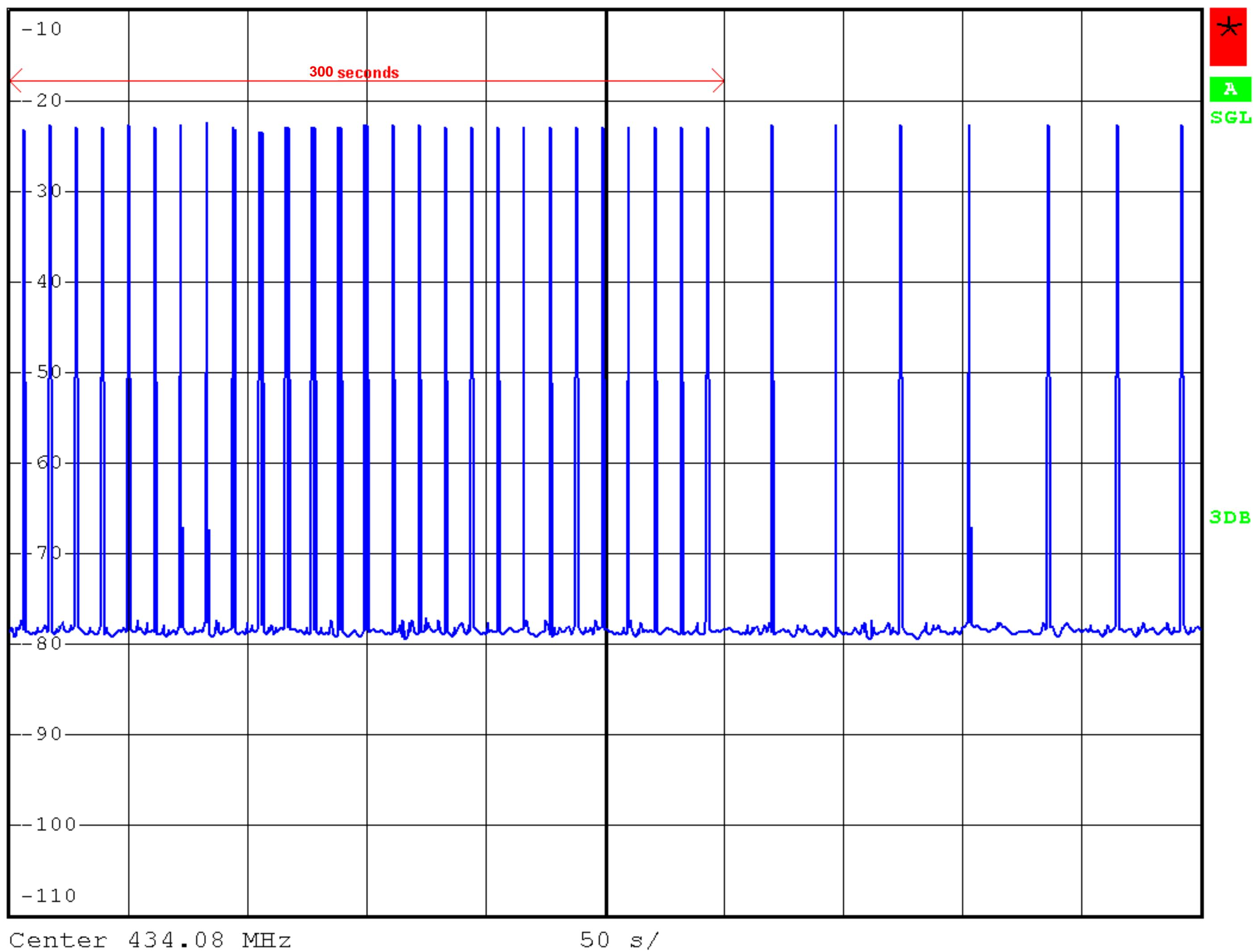
At the first 300 seconds, the EUT transmits every 11.0 seconds.
