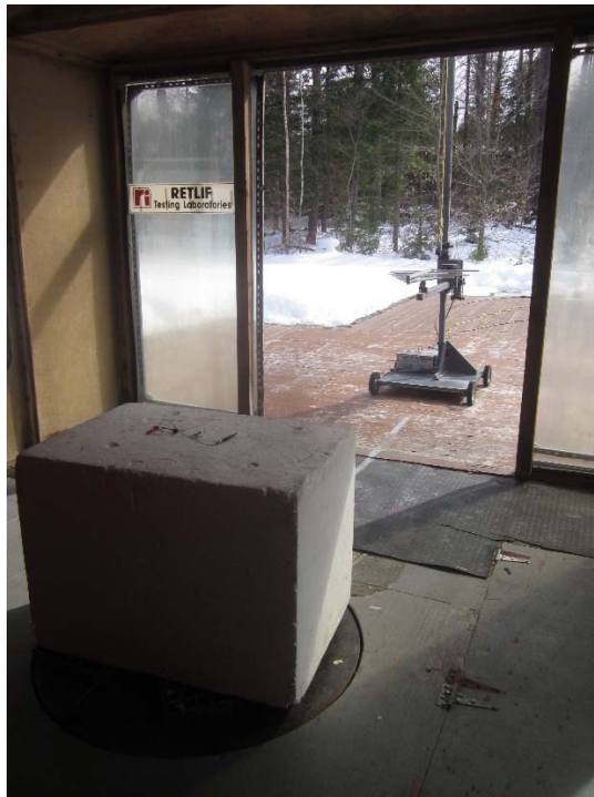
Horizontal Antenna Polarization, 200 MHz to 1 GHz, Log Periodic
