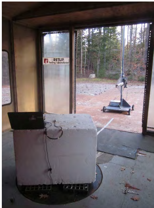
Vertical Antenna Polarization, Linx Antenna & 12" Cable Configuration, 200 MHz to 1 GHz, Log Periodic
