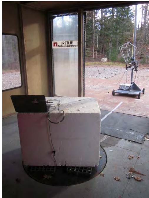
Vertical Antenna Polarization, L-Com Antenna & 1m Cable, 30 MHz to 200 MHz, Biconical Antenna
