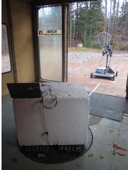
Vertical Antenna Polarization, Laird Antenna & 1 m Cable Configuration, 30 MHz to 200 MHz, Biconical Antenna
