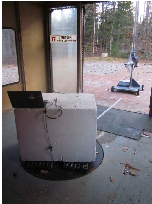
Vertical Antenna Polarization, Internal Antenna Configuration, 200 MHz to 1 GHz, Log Periodic
