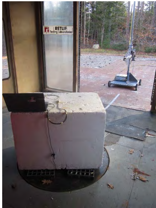
Vertical Antenna Polarization, Laird Antenna & 1 m Cable Configuration, 200 MHz to 1 GHz, Log Periodic
