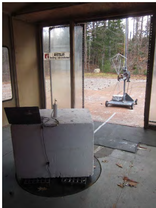
Vertical Antenna Polarization, MMCX Antenna Configuration, 30 MHz to 200 MHz, Biconical Antenna
