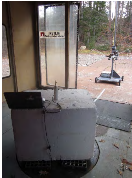
Horizontal Antenna Polarization, MMCX Antenna Configuration, 30 MHz to 200 MHz, Biconical Antenna
