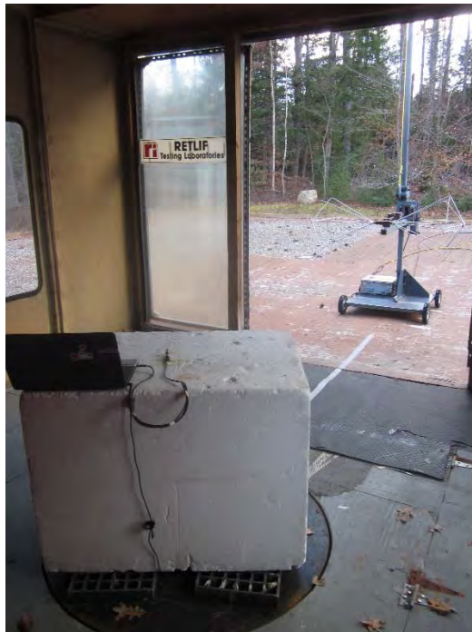
Horizontal Antenna Polarization, Internal Antenna Configuration, 30 MHz to 200 MHz, Biconical Antenna
