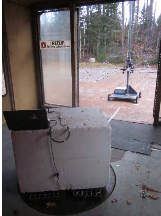
Horizontal Antenna Polarization, Laird Antenna & 1 m Cable Configuration, 30 MHz to 200 MHz, Biconical Antenna
