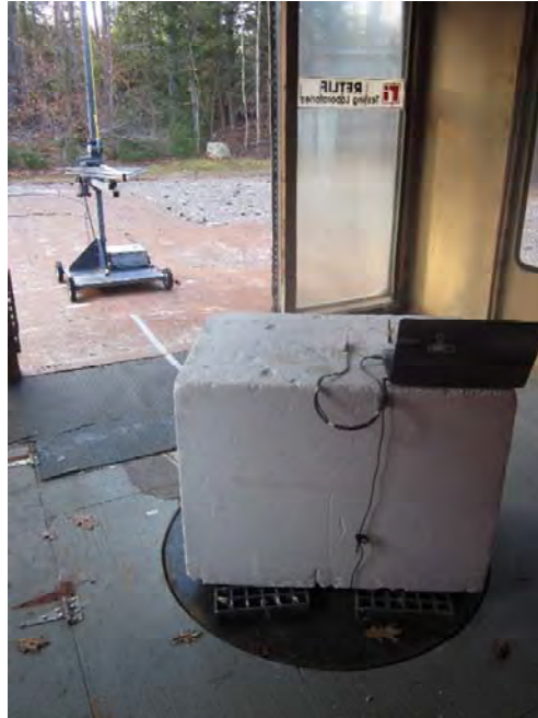
Horizontal Antenna Polarization, Linx Antenna & 12" Cable Configuration, 200 MHz to 1 GHz, Log Periodic
