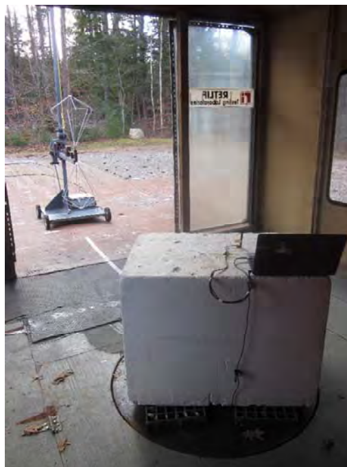
Vertical Antenna Polarization, Linx Antenna & 3" Cable Configuration, 30 MHz to 200 MHz, Biconical Antenna
