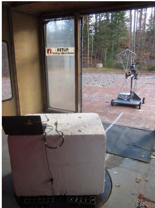
Vertical Antenna Polarization, Linx Antenna & 12" Cable Configuration, 30 MHz to 200 MHz, Biconical Antenna
