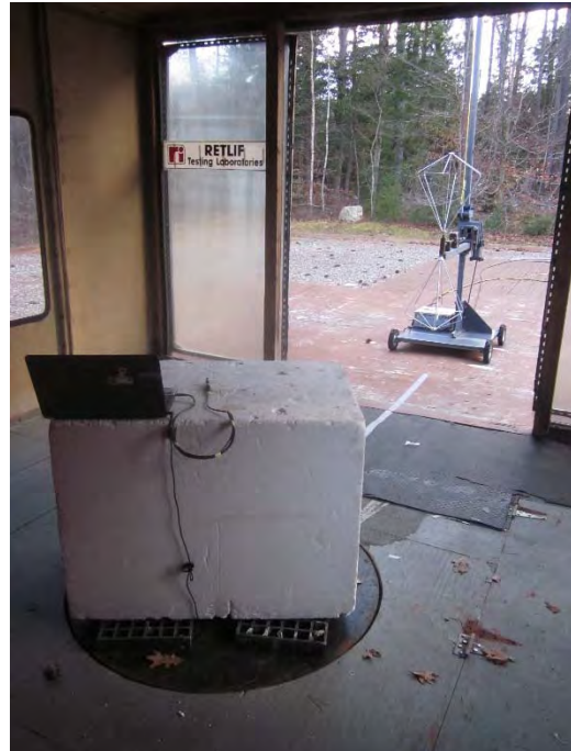
Vertical Antenna Polarization, Internal Antenna Configuration, 30 MHz to 200 MHz, Biconical Antenna
