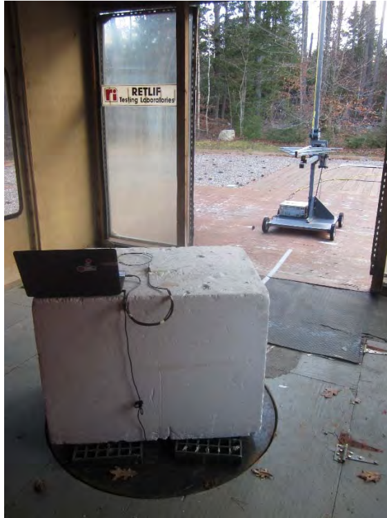
Horizontal Antenna Polarization, L-Com Antenna & 1m Cable, 200 MHz to 1 GHz, Log Periodic
