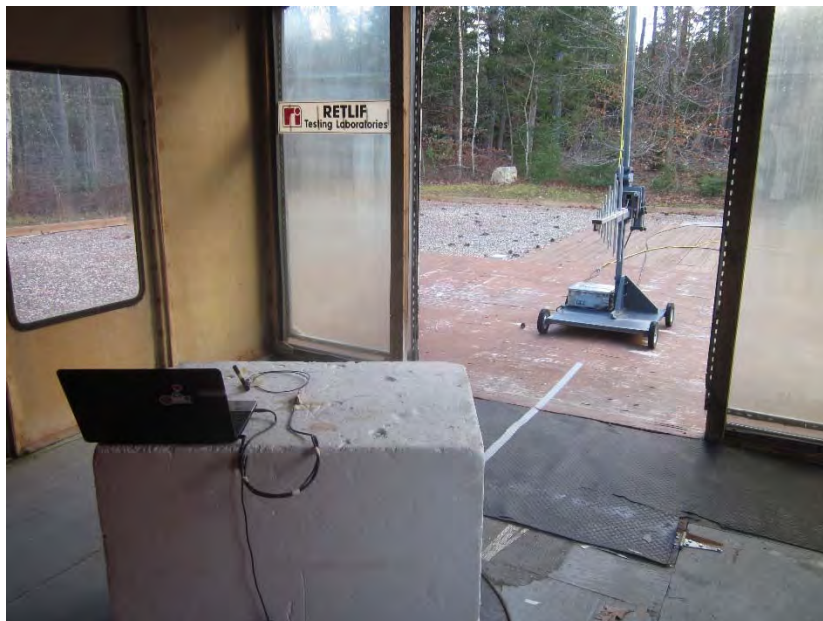
Vertical Antenna Polarization, L-Com Antenna & 1m Cable, 200 MHz to 1 GHz, Log Periodic
