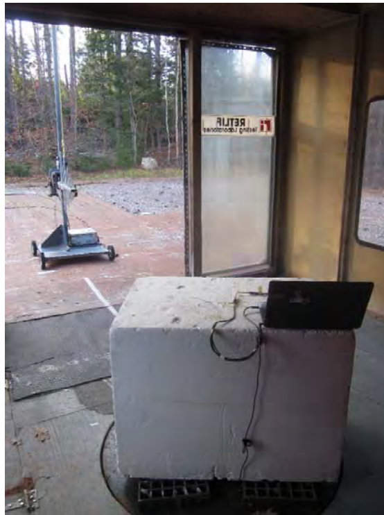
Vertical Antenna Polarization, Linx Antenna & 3 Cable Configuration, 200 MHz to 1 GHz, Log Periodic
