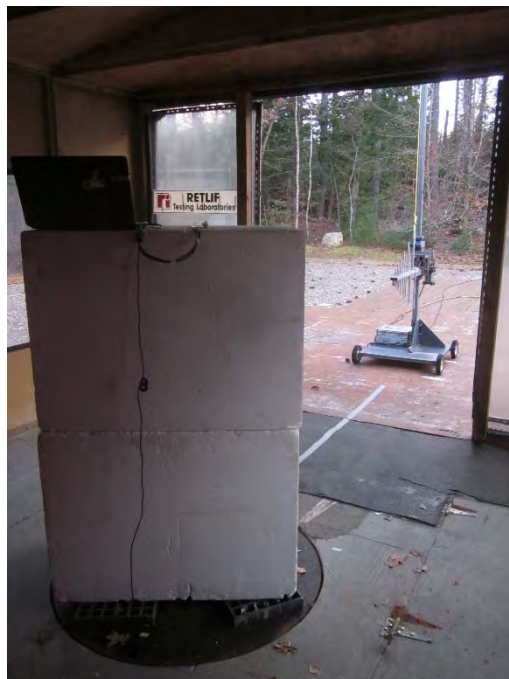
Vertical Antenna Polarization, MMCX Antenna Configuration, 200 MHz to 1 GHz, Log Periodic
