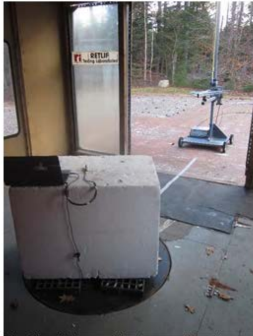
Horizontal Antenna Polarization, Internal Antenna Configuration, 200 MHz to 1 GHz, Log Periodic
