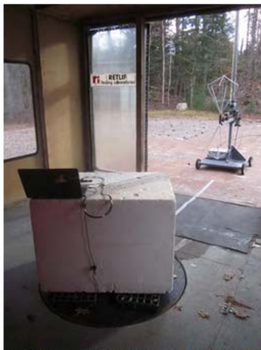
Vertical Antenna Polarization, L-Com Antenna & 1m Cable, 30 MHz to 200 MHz, Biconical Antenna
