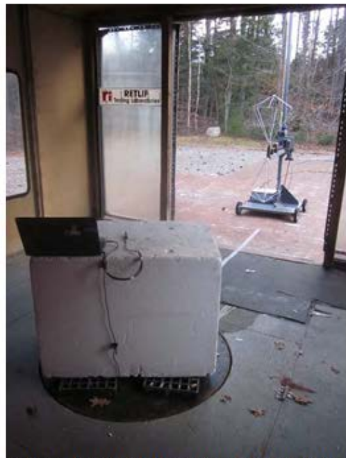
Vertical Antenna Polarization, Internal Antenna Configuration, 30 MHz to 200 MHz, Biconical Antenna
