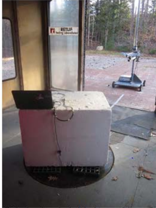
Horizontal Antenna Polarization, Laird Antenna & 1 m Cable Configuration, 200 MHz to 1 GHz, Log Periodic
