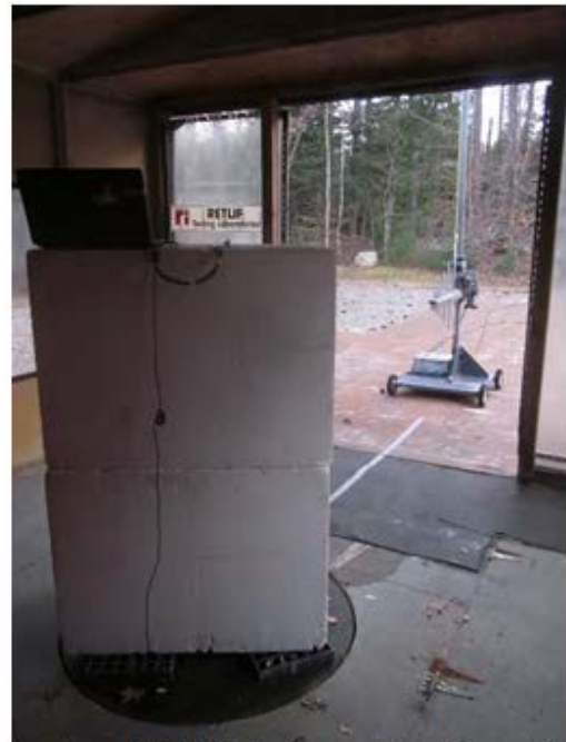
Vertical Antenna Polarization, MMCX Antenna Configuration, 200 MHz to 1 GHz, Log Periodic
