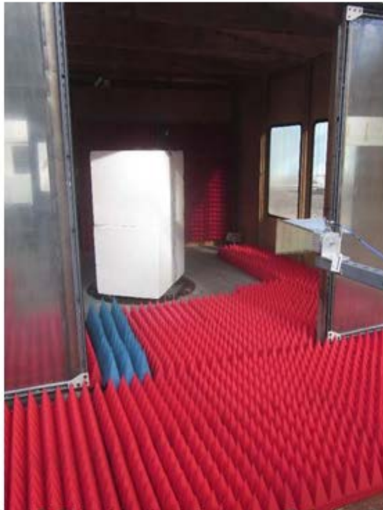
1 to 18 GHz, Vertical Antenna Polarization
