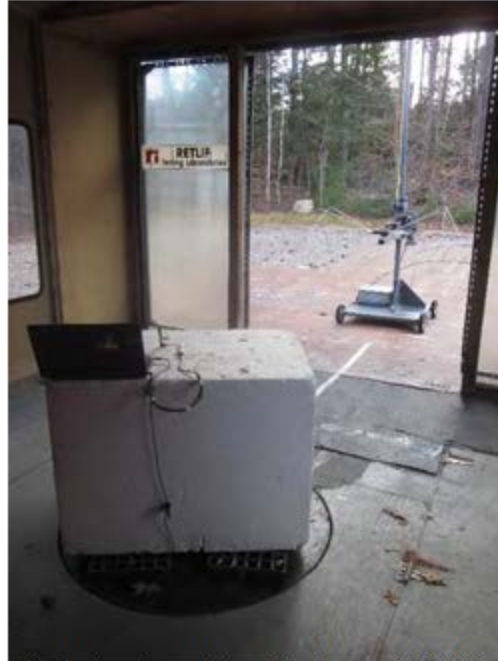
Horizontal Antenna Polarization, Linx Antenna & 3" Cable Configuration, 30 MHz to 200 MHz, Biconical Antenna
