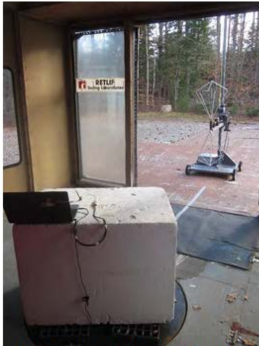
Vertical Antenna Polarization, Linx Antenna & 12" Cable Configuration, 30 MHz to 200 MHz, Biconical Antenna
