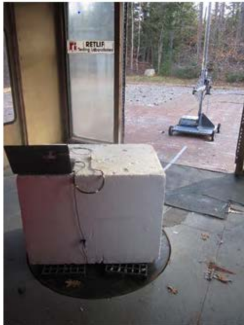
Vertical Antenna Polarization, Laird Antenna & 1 m Cable Configuration, 200 MHz to 1 GHz, Log Periodic
