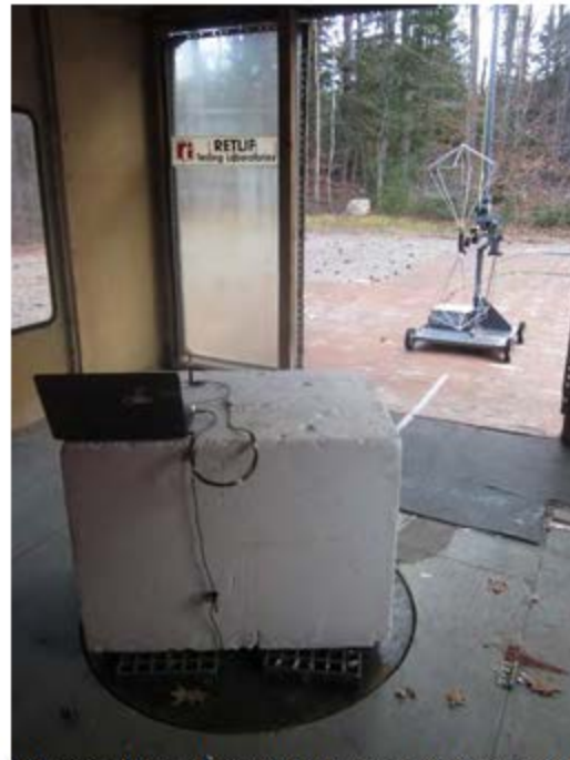
Vertical Antenna Polarization, Laird Antenna & 1 m Cable Configuration, 30 MHz to 200 MHz, Biconical Antenna
