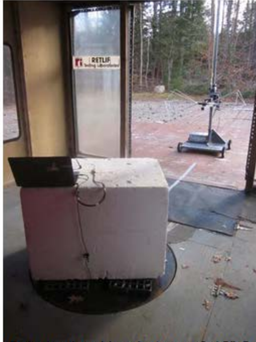
Horizontal Antenna Polarization, Linx Antenna & 12" Cable Configuration, 30 MHz to 200 MHz, Biconical Antenna
