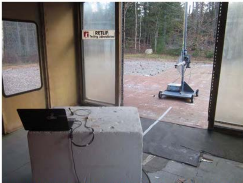
Vertical Antenna Polarization, L-Com Antenna & 1m Cable, 200 MHz to 1 GHz, Log Periodic
