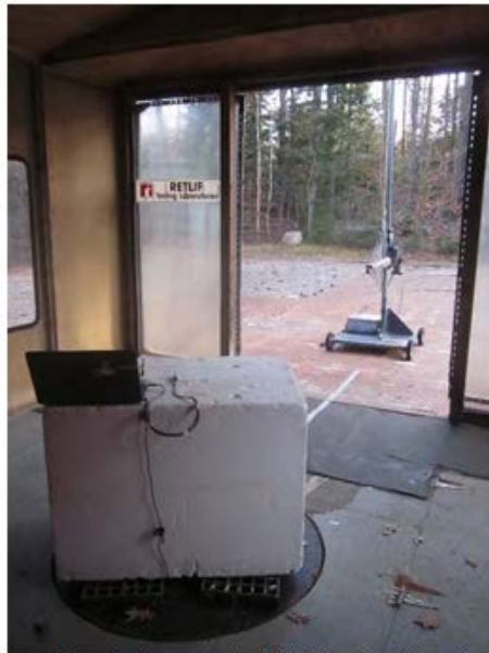
Vertical Antenna Polarization, Linx Antenna & 12" Cable Configuration, 200 MHz to 1 GHz, Log Periodic
