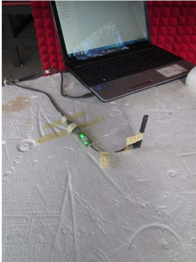
Linx Antenna & 3 m Cable Configuration
