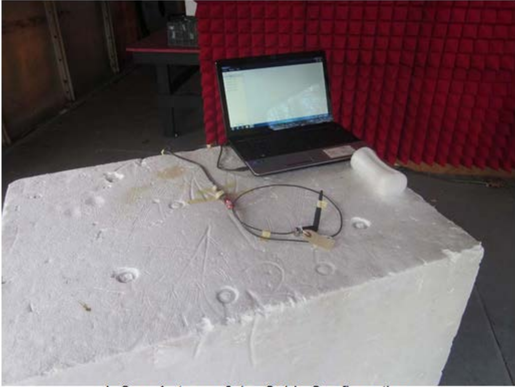
L-Com Antenna & 1m Cable Configuration
