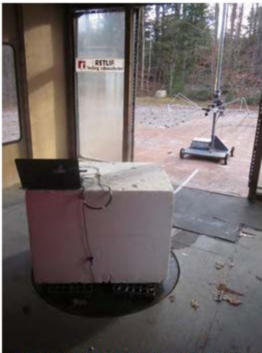
Horizontal Antenna Polarization, L-Com Antenna & 1m Cable, 30 MHz to 200 MHz, Biconical Antenna
