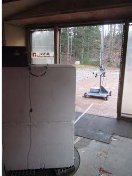
Horizontal Antenna Polarization, MMCX Antenna Configuration, 200 MHz to 1 GHz, Log Periodic
