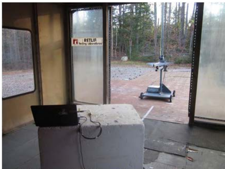
Horizontal Antenna Polarization, Linx Antenna & 3 Cable Configuration, 200 MHz to 1 GHz, Log Periodic
