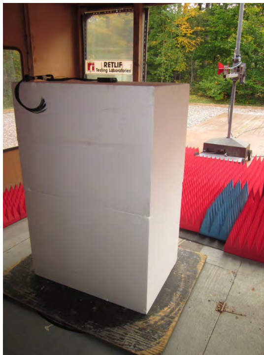
Horizontal Antenna Polarization, 1 GHz to 12 GHz, Internal Antenna, 150 cm
