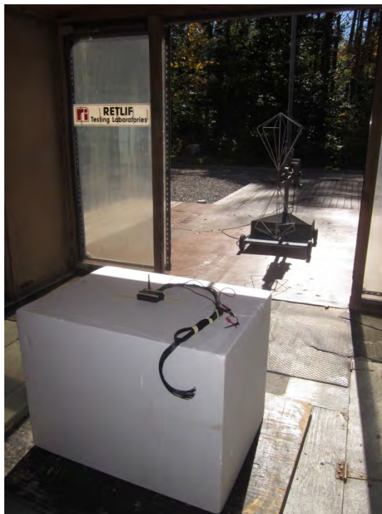
Vertical Antenna Polarization, 30 MHz to 200 MHz, External Antenna
