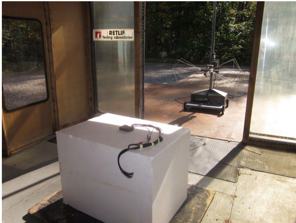
Horizontal Antenna Polarization, Internal Antenna
