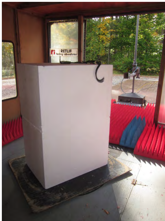
Horizontal Antenna Polarization, 12 GHz to 18 GHz, External Antenna, 150 cm
