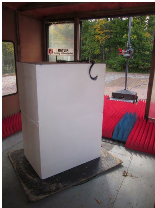
Horizontal Antenna Polarization, 1 GHz to 12 GHz, External Antenna, 150 cm
