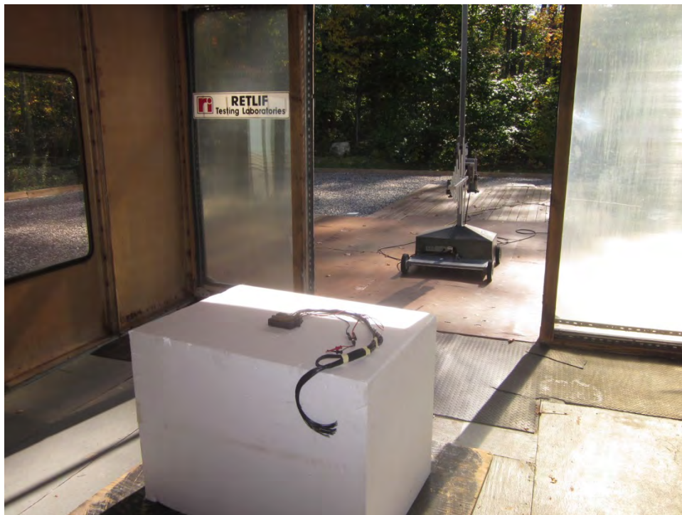
Vertical Antenna Polarization, Internal Antenna
