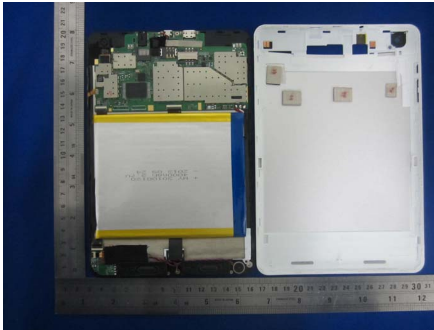
EUT- Rear Cover Off View
