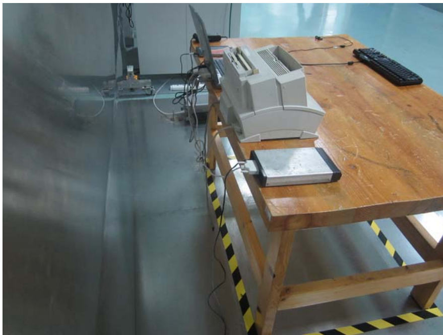
Conducted Emissions – Side View (Downloading Mode)
