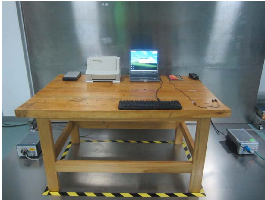
Conducted Emissions – Side View (Downloading Mode)
