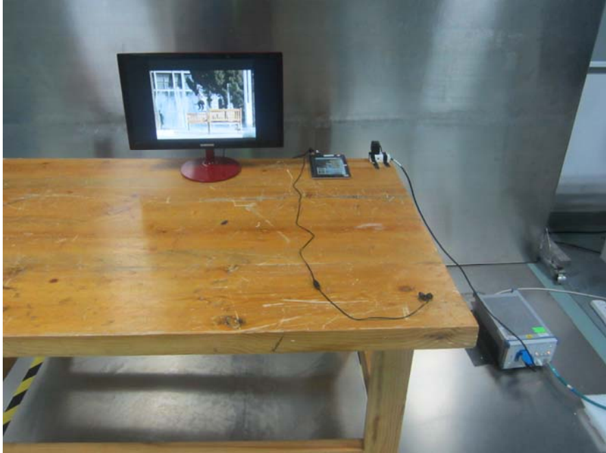
Conducted Emissions – Side View (Charging&Playing Mode)
