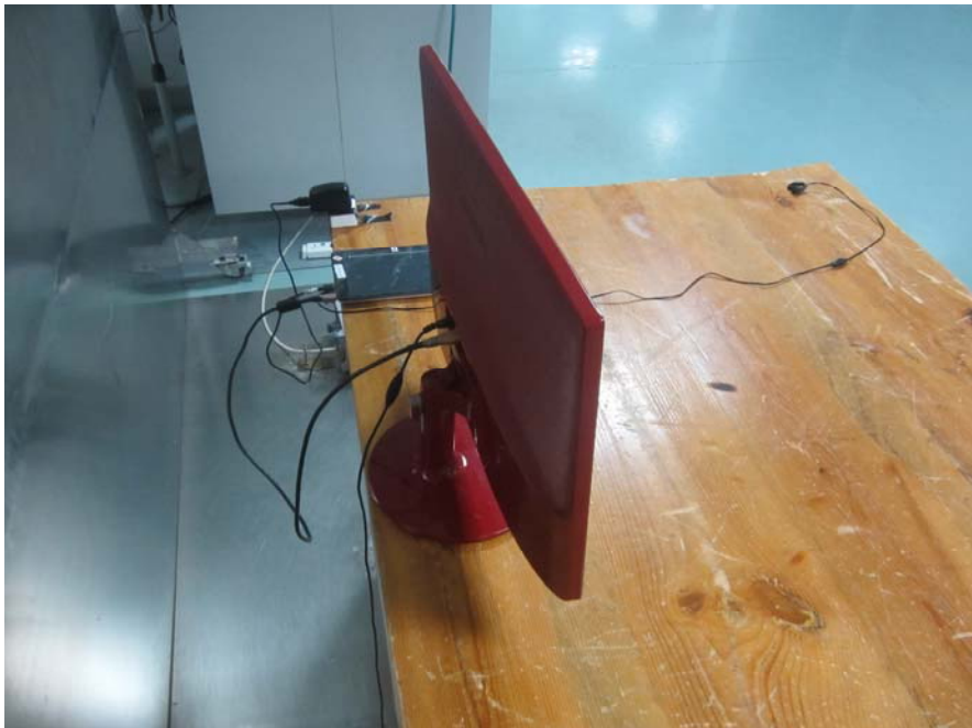
Conducted Emissions – Side View (Charging&Playing Mode)
