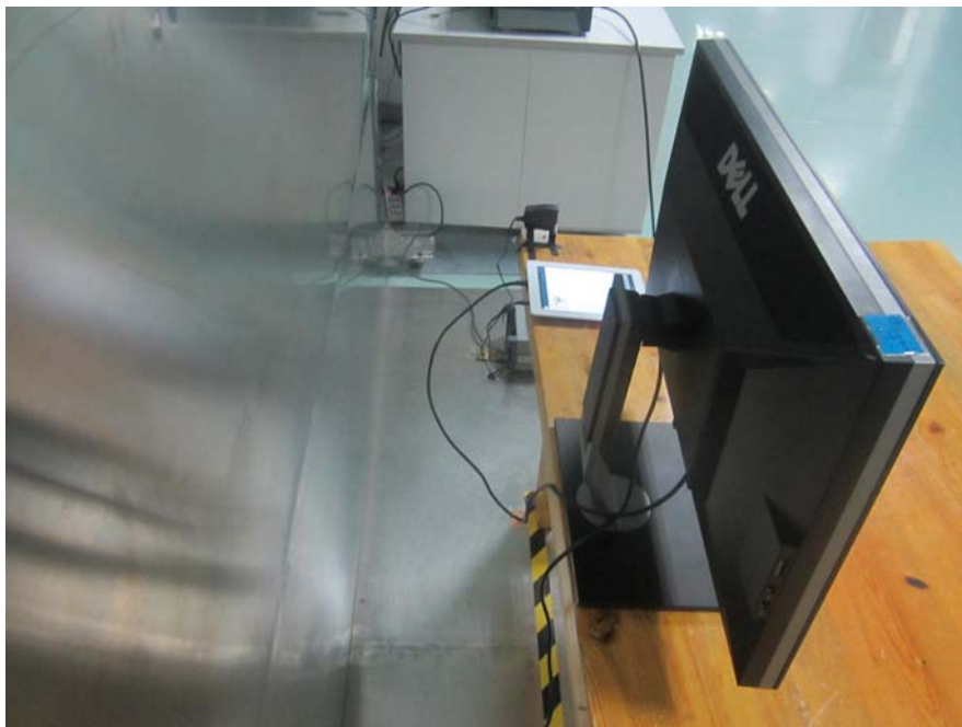
Conducted Emissions – Side View (HDMI Playing)
