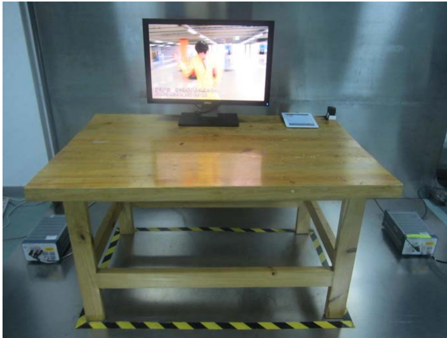
Conducted Emissions - Front View (HDMI Playing)
