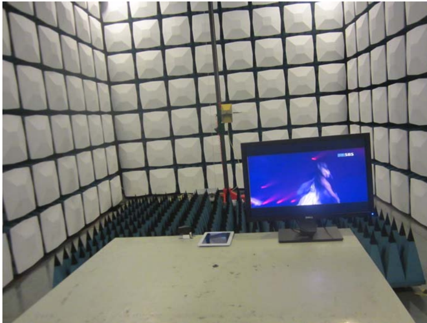
Radiated Emission -Front View (HDMI Playing) (Above 1GHz)
