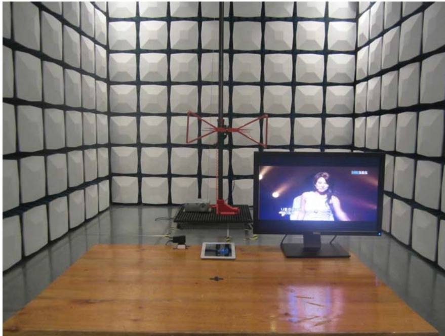
Radiated Emission -Front View (HDMI Playing) (Below 1GHz)
