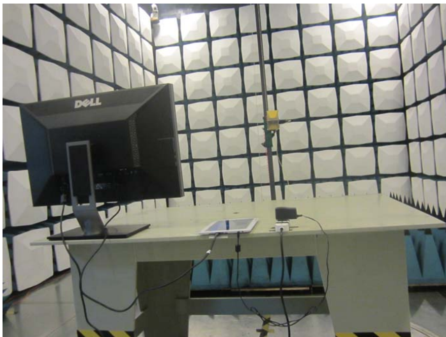
Radiated Emission - Rear View (HDMI Playing) (Above 1GHz)
