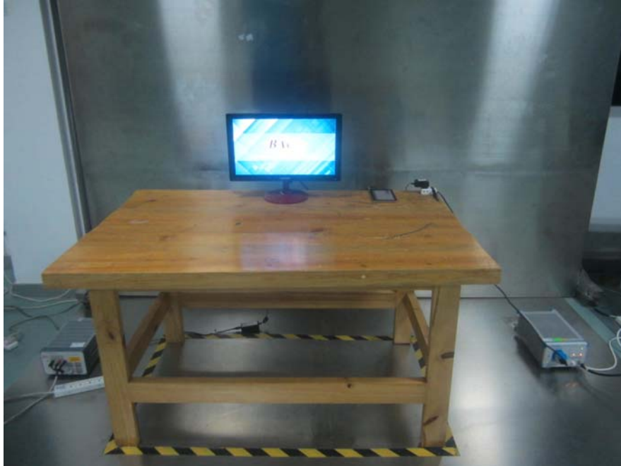
Conducted Emissions - Front View (HDMI Output)
