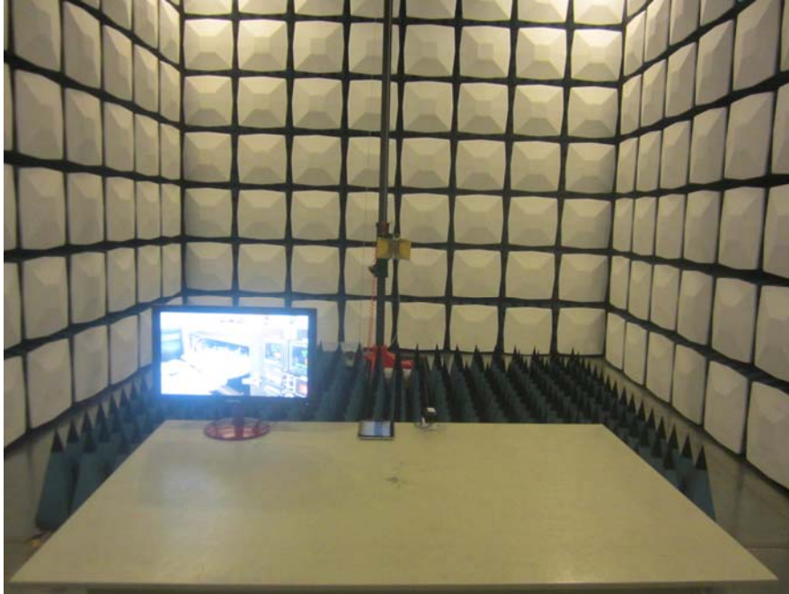
Radiated Emission - Rear View (HDMI Output) (Above 1GHz)
