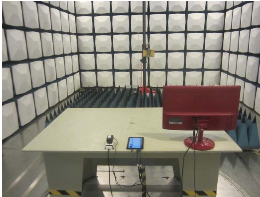
Radiated Emission - Rear View (HDMI Output) (Above 1GHz)
