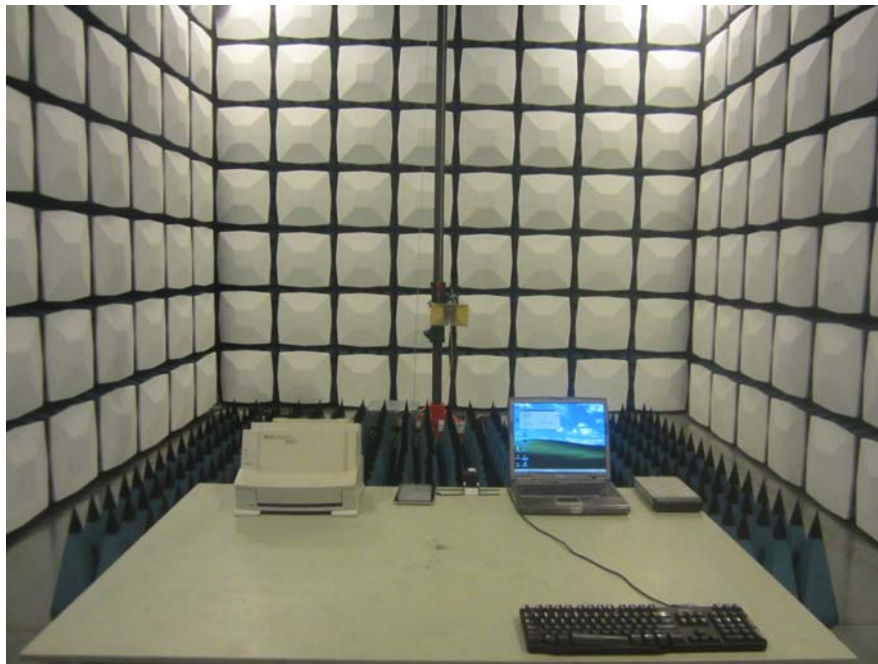
Radiated Emission - Rear View (USB Downloading) (Above 1GHz)
