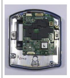
WPS LCD Frame and front cover assembly
