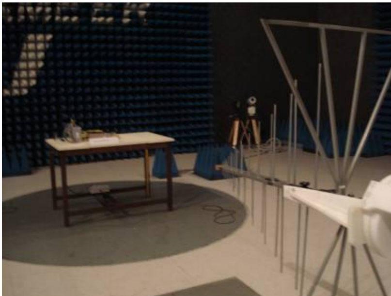
Radiated Emission Test Setup
