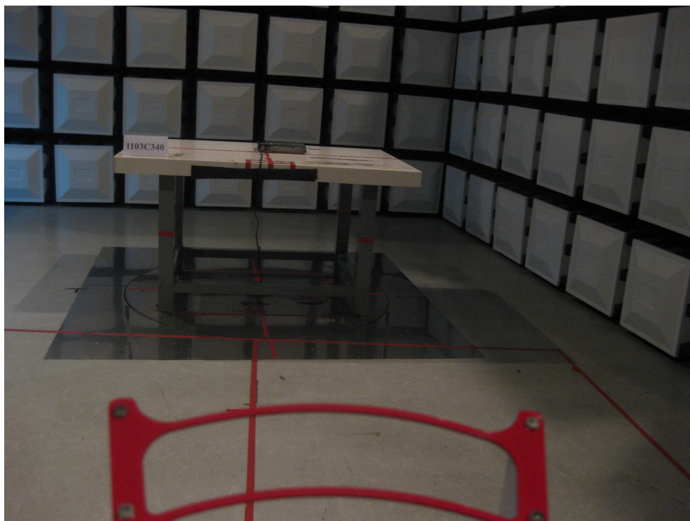
Photograph 3: Set-up for Radiation Measurement above 1GHz
