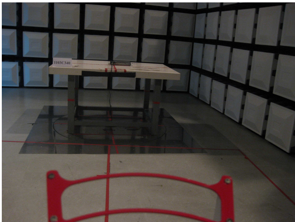
Photograph 3: Set-up for Radiation Measurement above 1GHz
