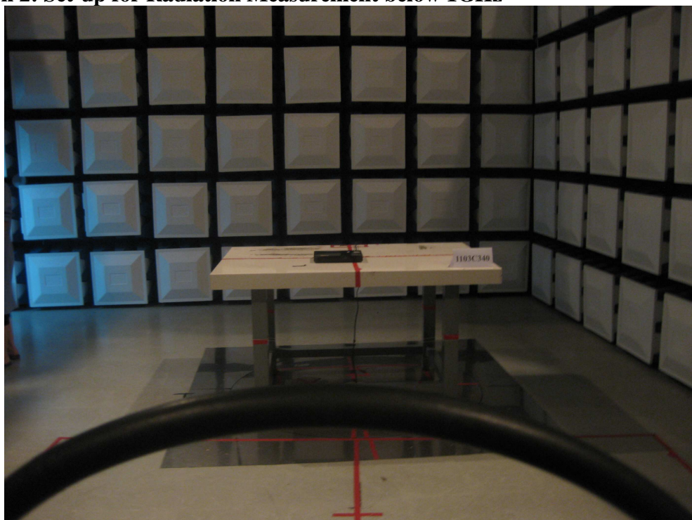
Photograph 2: Set-up for Radiation Measurement below 1GHz
