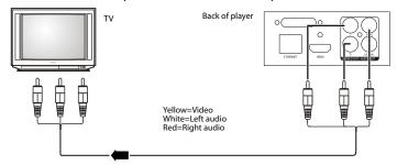
**Note**: The A/V cable can only send standard-definition video (480i) to
