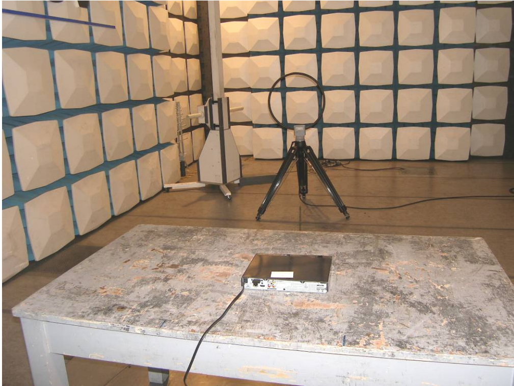
Photograph 2: Set-up for Radiation Measurement below 1GHz
