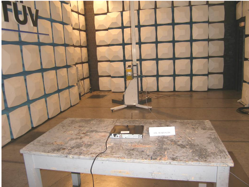
Photograph 3: Set-up for Radiation Measurement above 1GHz
