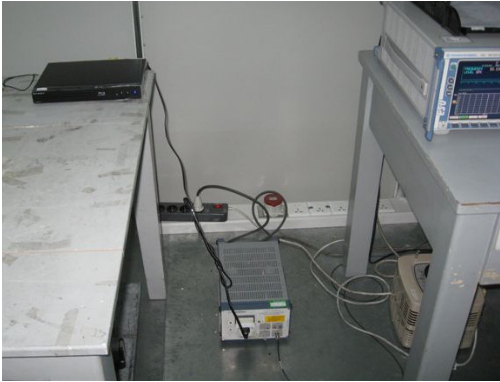
Photograph 1: Set-up for Conducted Emission Measurement
