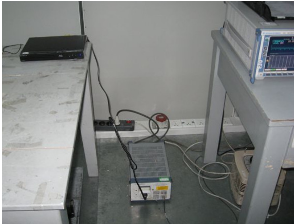
Photograph 1: Set-up for Conducted Emission Measurement
