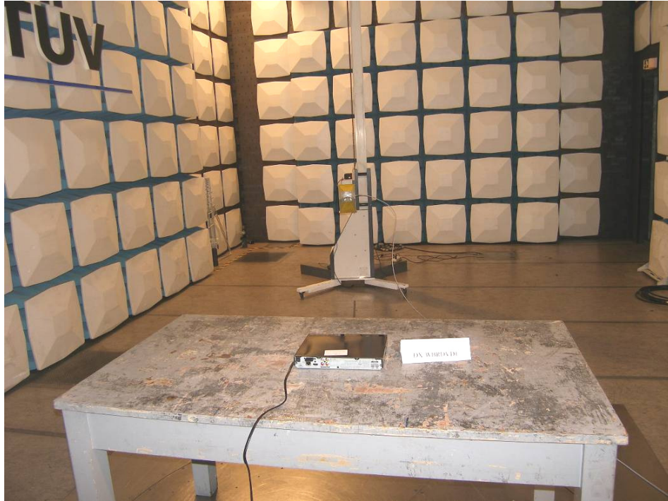
Photograph 3: Set-up for Radiation Measurement above 1GHz
