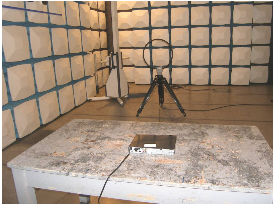
Photograph 2: Set-up for Radiation Measurement below 1GHz
