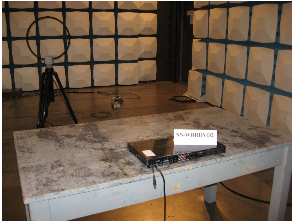
Photograph 2: Set-up for Radiation Measurement below 1GHz
