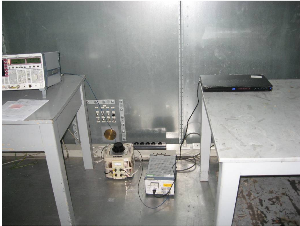
Photograph 1: Set-up for Conducted Emission Measurement
