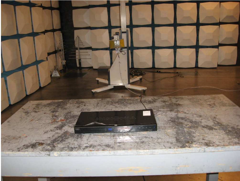
Photograph 3: Set-up for Radiation Measurement above 1GHz
