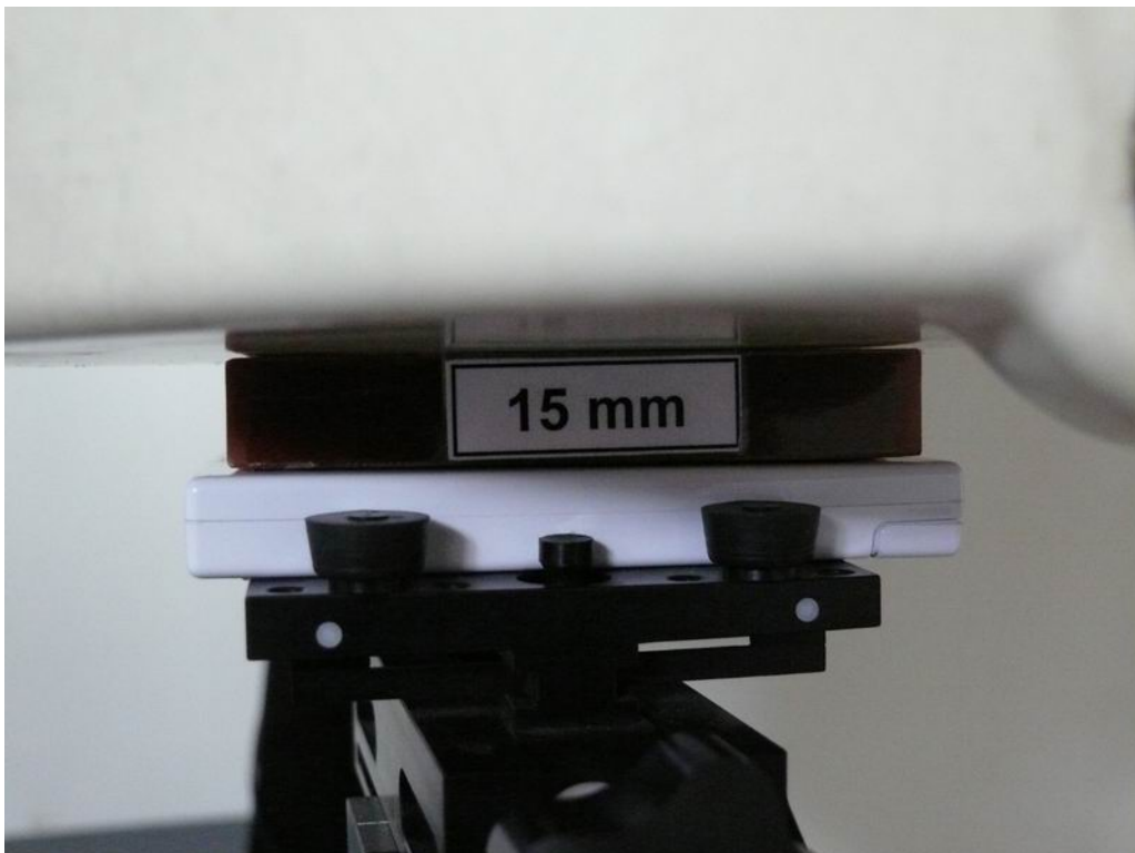
Picture 12: Body, The EUT display towards phantom, the distance from handset to the bottom of the Phantom is 15mm
