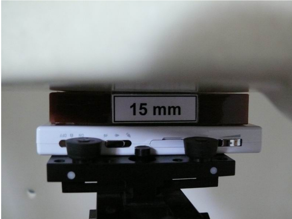
Picture 11: Body, The EUT display towards ground, the distance from handset to the bottom of the Phantom is 15mm
