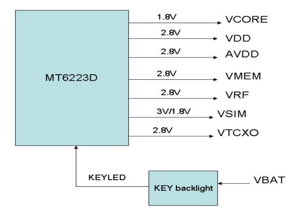
MT6223D includes 7 LDOs and KEY backlight control block and it can
