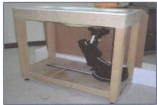
Figure 5 Generic Twin Phantom
