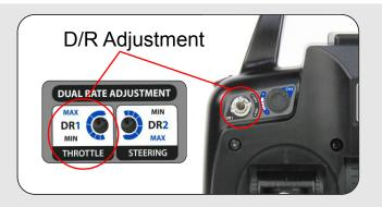
**Note** - When using electronic ESCs on CH1 or CH2 it is essential that the switches are in the Off position when powering the transmitter and the receiver. This allows the ESCs to calibrate correctly.
