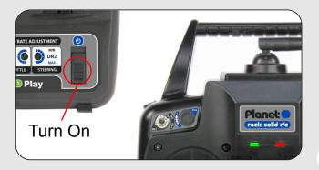
Turn on the receiver power and note the receiver LED will illuminate a solid red. This indicates it has successful paired with the transmitter.
