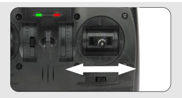
To adjust the centre point of the receiver CH2 output, hold the trim button on the left gimbal up or down as needed.
