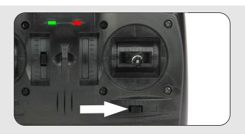
To reverse CH2, power off the Tx. Hold the trim on the left gimbal up and turn the TX power back on. Keep holding the trim up until the green LED goes solid. Release the trim button and check for correct operation.
