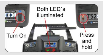
Keep holding the transmitter Pair button until the receiver LED is extinguished. When the LED has extinguished release the transmitter Pair button.
