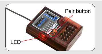
Turn on the transmitter power. As soon as the red and green LEDs are illuminated press and hold the Pair button.
