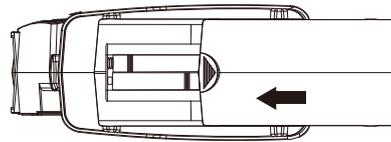
1. Press down on the battery cover and slide in the direction of the arrow to remove.
