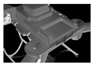
• There are plug pins under & above the Quad-copter, which are for connecting to the Camera gimbal controls, Video in/out, external servos, OSD unit, Video remote control....etc, no modification needed, just plug & play.
